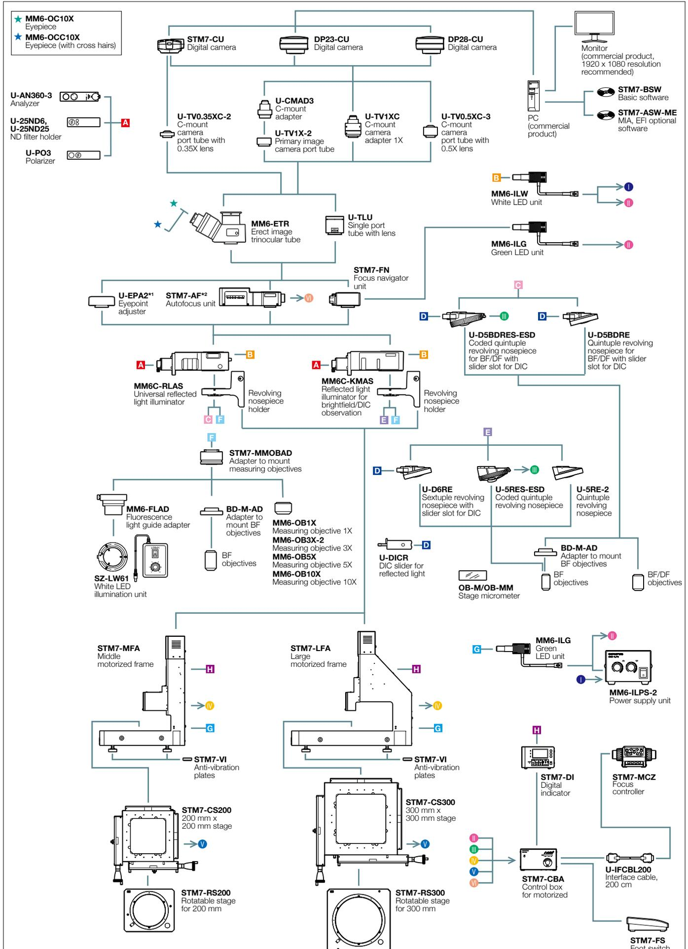
\*1 STM7-LFA frame combination only. Max. two mountable. \*2 STM7-AF autofocus unit is a Class 1 laser product.
