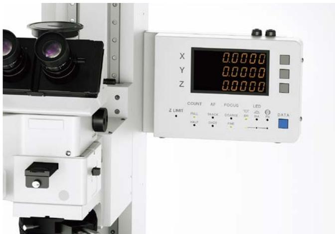
Digital readout attached to the frame
